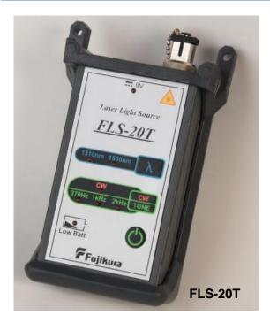
The FLS-20T is rugged and compact designed Laser Light Source, which is used for optical fiber testing. The FLS-20T generates the laser light at wavelength of 1,310nm and 1,550nm selectable for singlemode fiber. The mode of light signal is selectable from CW light and kinds of of modulated tones.
