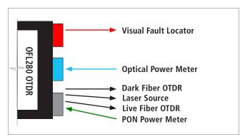
a. Adds ability to perform OTDR and loss tests at 1490 nm. However, testing at 1310 and 1550 nm is recommended and generally is all that is needed to test or fault-locate inactive (dark) FTTx PONs during construction.
