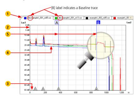
The Trace graph window displays OTDR test results in a graph format. Up to six traces can be displayed. The major features of the Trace graph window are explained below.
