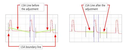
To adjust LSA lines, position the mouse pointer over an LSA line boundary, then click and drag to the desired location.
