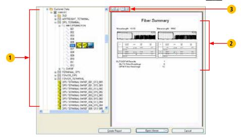
The Results Explorer application provides a brief preview of results within Results Explorer screen. Use this application to navigate test results, switch between OTDR and OLTS test viewers (when applicable), and access the Report Wizard as needed.
