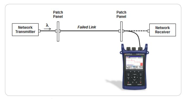
Figure 1: Out-of-service point-to-point link may be connected to an active transmitter.
