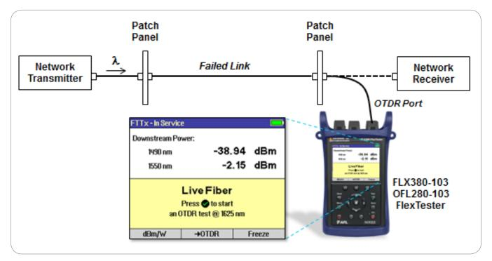
Figure 5: "Live Fiber" detected and displayed when OTDR test initiated on active fiber.
