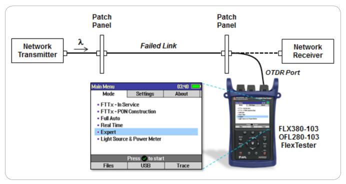
Figure 4: Connect fiber-under-test to OTDR port and select Full Auto or Expert mode.
