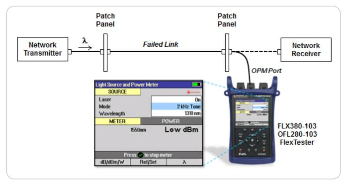
Figure 3: "Low" power level indicates fiber-under-test is dark.
