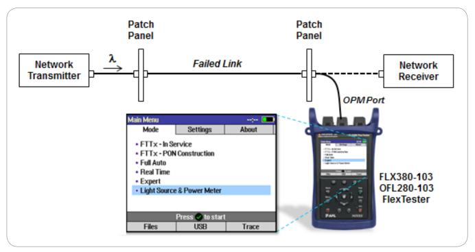
Figure 2: Connect Fiber-under-test to OPM Port and select "Light Source and Power Meter".
